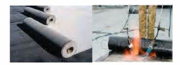
SBS Modified membrane is a special, SBS modified torch-on bituminous membrane. The multilayered membrane consists of non –woven polyester, both sides coated with elastomeric rubber modified bituminous compound. This coating will provide stability in various climatic conditions.
