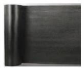
Protection Membrane is an APP modified bituminous Prefabricated Protection membrane strengthened by Non–Woven Polyester mat. The multilayered structure with an exceptionally formulated Polymer modified bituminous Compound will provide high Puncture &Impact Resistance for water proofing system.
